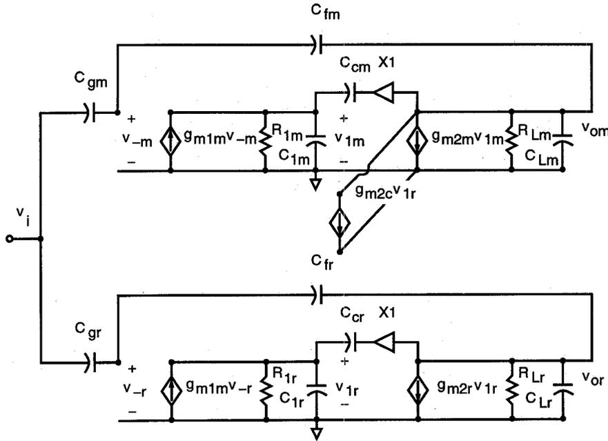
Fig. 12. Small signal model of a two-stage op amp.
