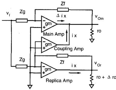
Fig. 3. A replica-amp gain-enhancement technique.
