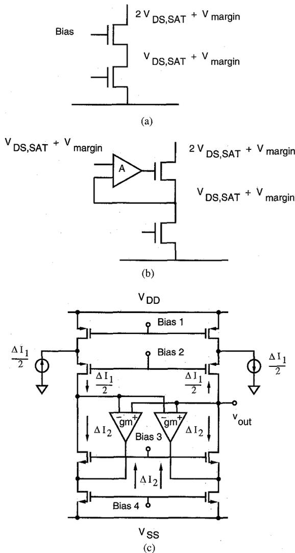
Fig. 1. Conventional gain-enhancement techniques. (a) A regular cascode circuit. (b) An active cascode circuit. (c) A positive feedback circuit.
