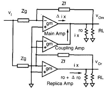
Fig. 5. A moderate resistive load does not degrade effective open-loop gain.
