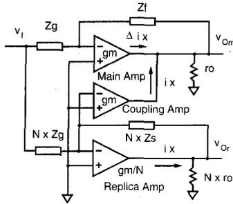
Fig. 4. Minimizing power and area by scaling down the replica amplifier.
