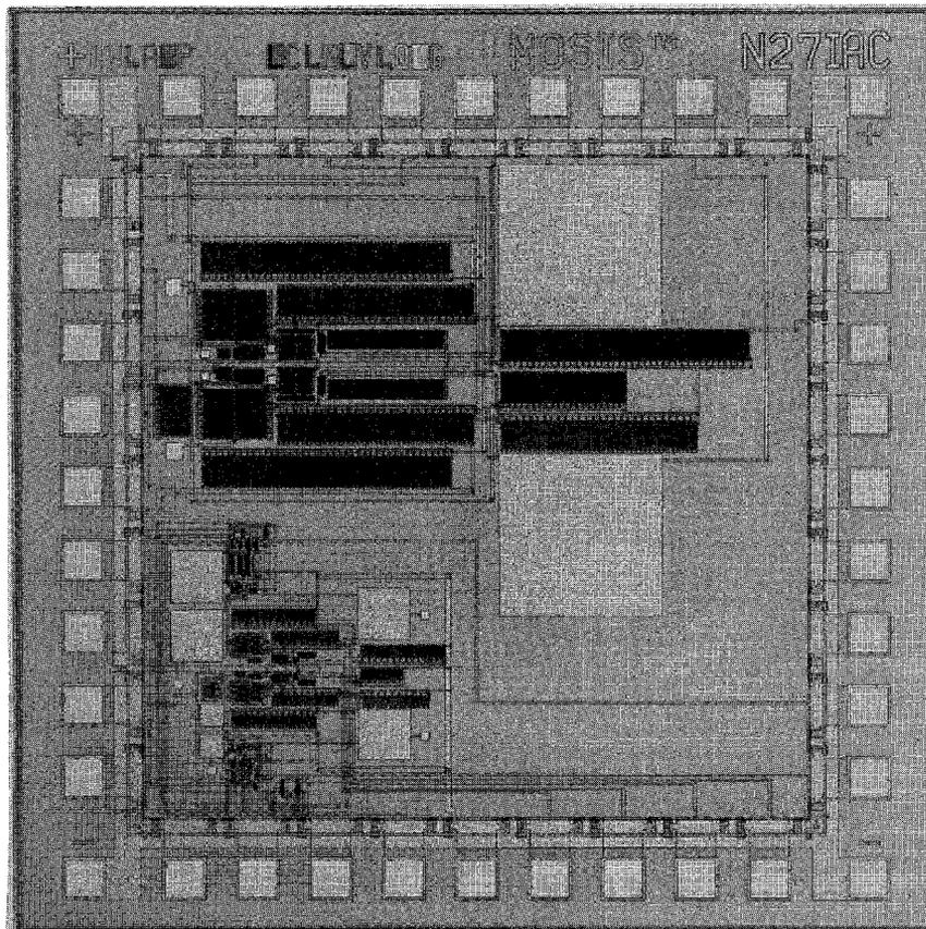
Fig. 11. Chip photograph of the two-stage op amp.
